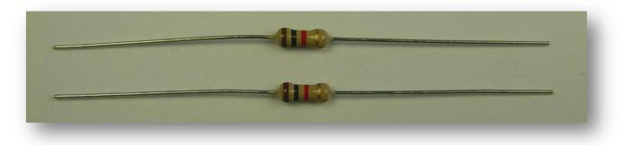
Photo 2. Resistors R1 and R4 are  $1K\Omega$  (one thousand ohms), with brown, black and red stripes.
