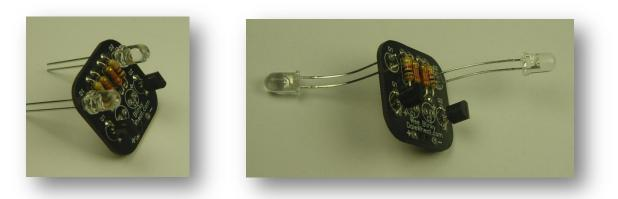
Photo 14. LEDs inserted flush against PCB.
