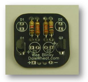
Photo 11. The transistors have been installed correctly.
