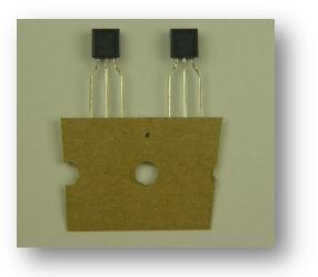
Photo 8. Transistors on tape.
