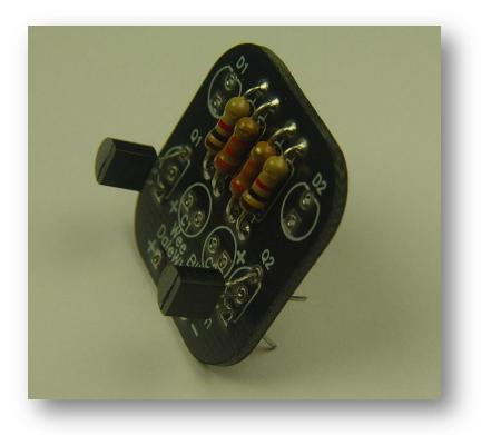
Photo 10. The correct way to insert the transistors.
