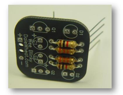
Photo 5. Insert the resistors into the PCB. Make sure you put the right resistor in the right place.
