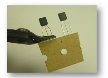
Photo 9. Cut the transistor leads near the edge of the tape. Don't try to remove the tape from the leads.
