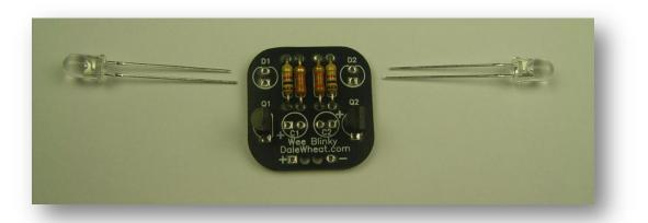
Photo 13. The long lead, or *anode*, goes in the hole with the square pad. It won't work the other way.
