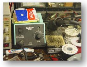
Use a small gauge solder that contains flux. Almost anything will do. You can use lead-free solder if you want but I'm hearing rumors that there are long-term reliability problems with lead-free solder.
