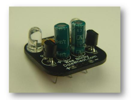
Photo 19. The capacitor cathode markings should be facing each other.
