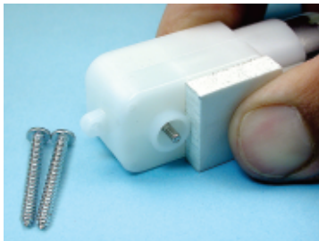
Aligning block to motor collar & tabletop. Put screws in through motor holes on the other side.
