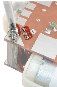
...Flip the PCB on, matching the holes for the pins, and screw together...
