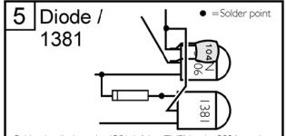
Solder the diode to the 1381 <code>left leg, THEN</code> to the 3906 transistor as shown, with the 1381 <code>middle leg</code> connected to the 3906 <code>left leg, and the 1381 <code>left leg</code> connected to the 3906 <code>right leg.</code></code>
