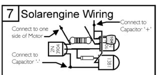
Now your Symet Solarengine is ready to connect to the rest of the Symet. Use these electrical connection points to install it. Remember to watch for touching wires that might short it out!
