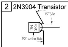
Bend the right side lead  $90^\circ$  up, so it points at you. Bend the left side lead  $90^\circ$  to the left side.
