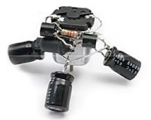
4) Skip ahead, and build your solarengine circuit. When done, install it tight to one side of the motor. The right leg of the 3904 goes to the other motor connection tab, the 3904 left leg solders to the motor body ('-'), and the left leg of the 3906 solders to any point of the '+' ring.
