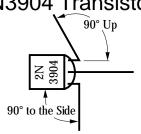
Bend the right side lead  $90^{\circ}$  up, so it points at you. Bend the left side lead  $90^{\circ}$  to the left side.
