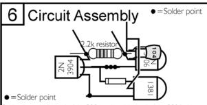
Solder the *middle lead of the 3904* to the *right lead of the 3906* with about 5mm (3/8") overlap. Solder the *right leg of the 1381* to the *left leg of the 3904*. Solder the resistor across the two vertical legs, and trim the excess off.
