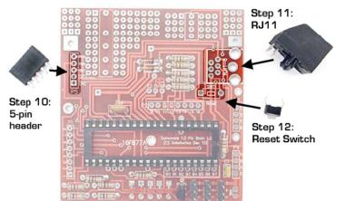
The single-pole, single-throw (SPST) microcontroller reset switch is installed at location 'SWT1'. Nothing to mysterious here!
