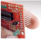
Remelt solder on top pin, and re-adjust pins so they sit properly, then solder the rest of the pins
