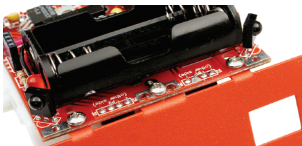
Screwing the plate on with 3 thread-forming screws
