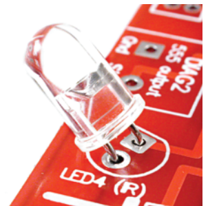
IR LED Installation
