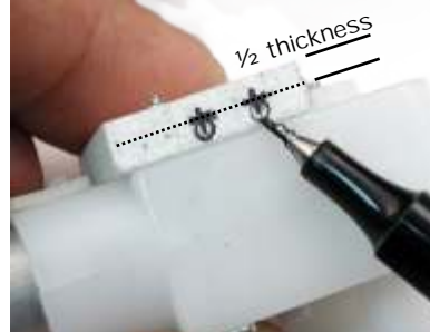
18d. Inspect / move hole marks
