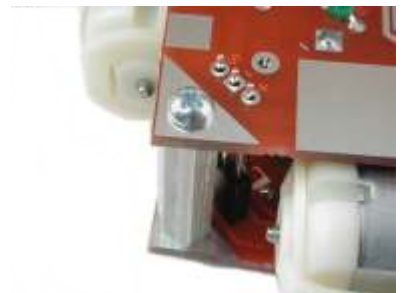
...So the screw pushes the pins down nice and even. Now solder the pins!
