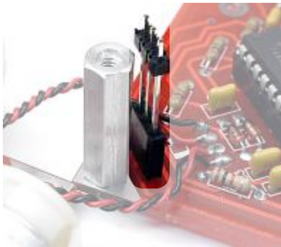
Insert 3-pin set into socket...
