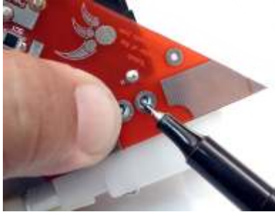
18c. Flip assembly, mark two screw holes
