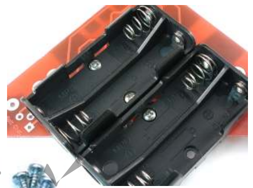
#2 x 3/16" Thread-forming screws. See? No pointy-tips!
