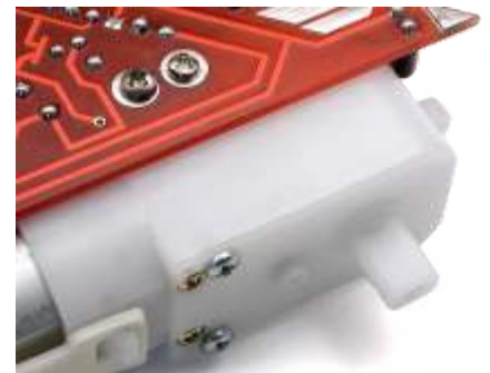
18f. Screw motor mount to PCB! Repeat for other motor.
