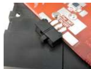
Switch installed properly
