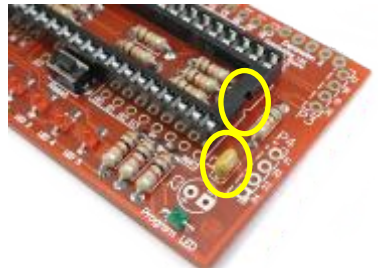
Finished installation of DIP carrier & 0.1 \mu F capacitor (note notch location on DIP carrier!)
