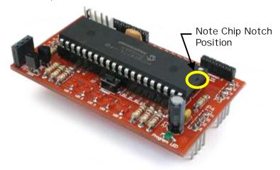
Having trouble getting the Microcontroller installed in the carrier? Try this: Gently bend all the chip pins inwards on a flat surface.
