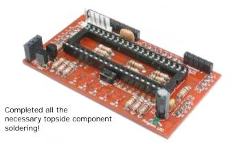
You're almost done. Let's flip the PCB over, and work entirely on the other side to install the mounting pins.
