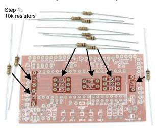
R1, R2, and R5 are used for RS-232 shift-levelling.
