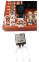
Close-up of the transistor installation
