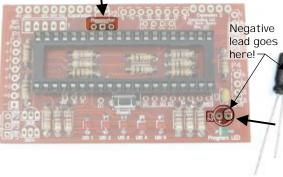
Step 10: 22µF capacitor. Note that the short leg near the stripe is installed in the negative pad!
