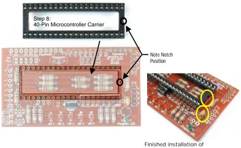
DIP carrier & 0.1µF capacitor (note notch location on DIP carrier! Steps 9, 10, 11
