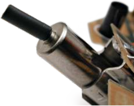
Cut a 6mm (1/4") length of heat-shrink tubing and stick it on the end of the motor shaft
