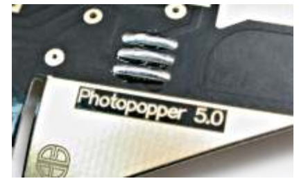
...solder it down, and snip the leads
