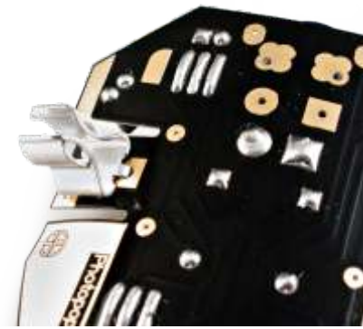
Left motor mount installed. Note tab position!
