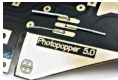
Fold the leads over on the topside...
