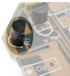
Note how the curve of the IR sensor matches the curve on the circuit board. With this many pictures, you should have nooo problem!
