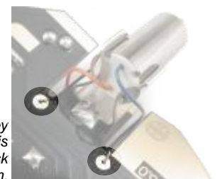
Run the red with under to the 'M-Red' pad, and the blue wire under to the 'M-Blue' pad
