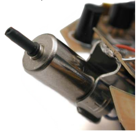
Trim it so there is about 1.5mm (1/16") left on the end. Now do it for the other motor!
