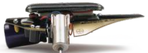
Much better. Sitting on just 2 motors and the main storage capacitor!
