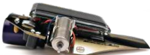
Too flat! Photopopper is doing belly-scrapes!
