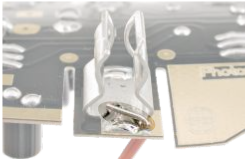
Insert the wire from underneath and lay it next to the motor clip
