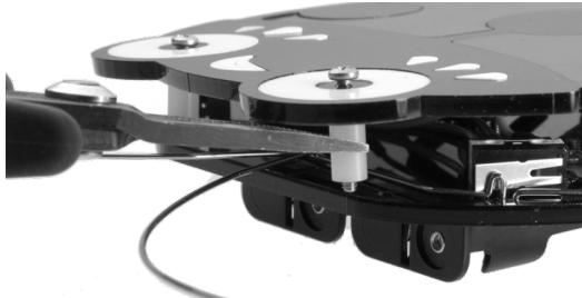
Step 13b - Put a screw in through the top, and a spacer underneath
