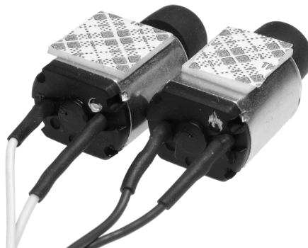
6b: Find the white dots on the motors, and stick the DSST on the side nearest the dot
