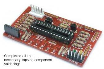
You're almost done. With the exception of the expansion sockets (later), you're done on the top-side. Let's flip the PCB over, and work entirely on the other side to install the mounting pins.
