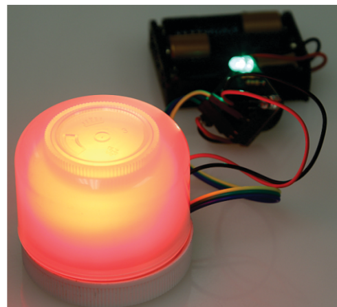
RGB Star mounted solo in Diffuser
