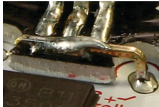
7c: Solder short leg into PCB
