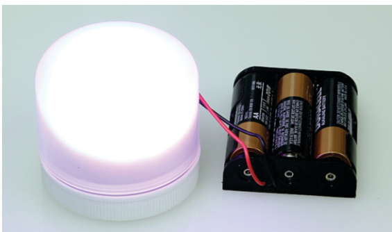
Diffuser container containing FireFly and RGB Star controller seen above
