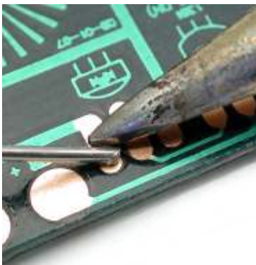
1. Presolder the pads...
