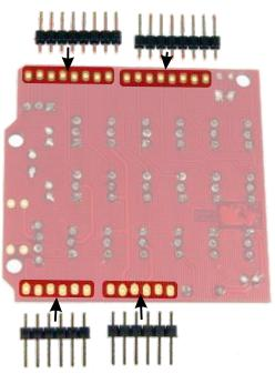
You are finished! Plug your SB-GVS shield into your Arduino / Freeduino, and you'll have a whole board to attach sensors to! We have tutorials and sample code on Solarbotics.com for this shield, so check if you are not sure what to do with it, check out our examples!
