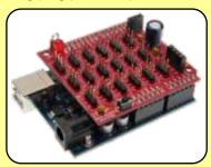
SB-GVS Shield on Arduino
