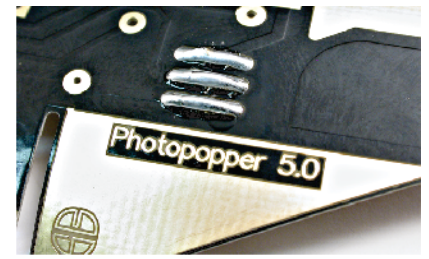
...solder it down, and snip the leads
