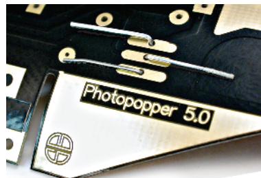
Fold the leads over on the topside...
