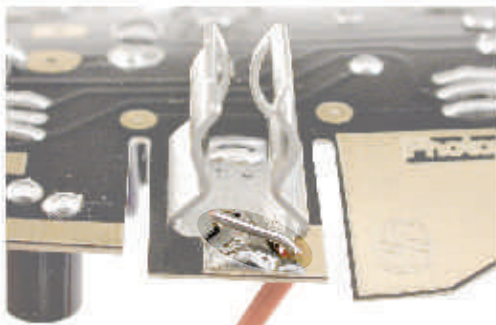
Insert the wire from underneath and lay it next to the motor clip
