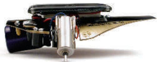
Much better. Sitting on just 2 motors and the main storage capacitor!
