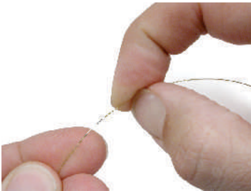
Form a curve by pinching the wire between your thumbnail and index finger, and pulling it through
