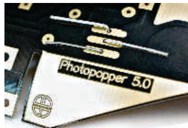
Fold the leads over on the topside...
