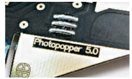
...solder it down, and snip the leads
