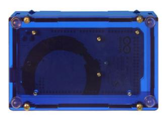
Mounting bolts thread into the acrylic and protrude a little out of the bottom, but the rubber feet more than compensate for them.
