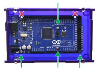
Place mounting bolts in the indicated locations, as they won't fit where the 'X's are, due to the headers.
