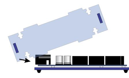
Assemble the 4 walls, and install the set by slipping the faceplate over the USB jack and power switch *first*.
