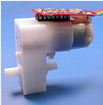
The GM2 installation - note the clipped motor retainer under the PCB
