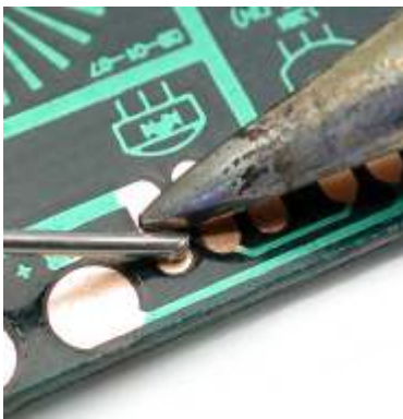
1. Presolder the pads...
