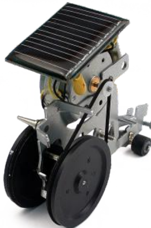
Ok, ok - we cheated a little . We had a spare mechanism, and found that we could push a second black wheel onto the same shaft as the main black wheel. And BOY does this little Solaroller zoom!
