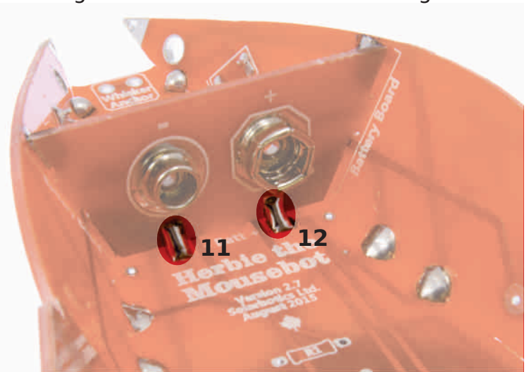
6B: The last 2 of the 12 solder points
