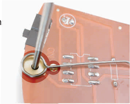
15A: Lay ring over spring, and note where you have to fold the wire down to meet the solder pad
