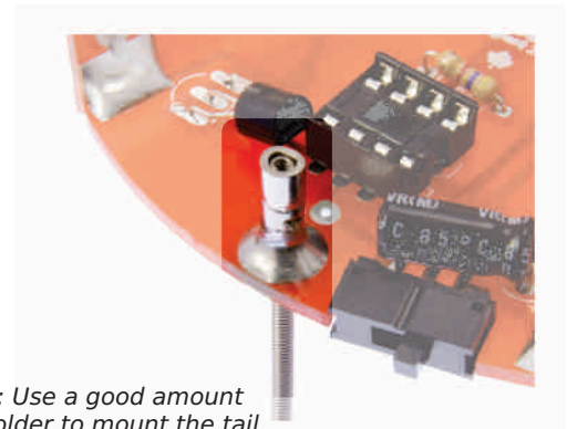
13B: Let the tail dangle underneath while soldering
