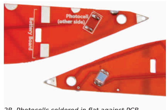
2B. Photocells soldered in flat against PCB
