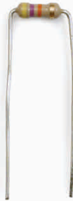
9A: Bend the 4.7k resistor (marked yel / pur / red) leads 90° down
