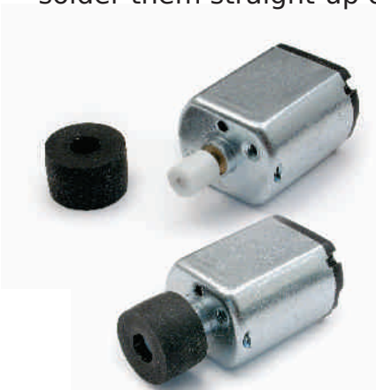
16A: Slide the rubber tire onto the motor's white hub
