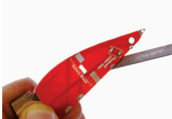
1B. Filing down the tab grooves
