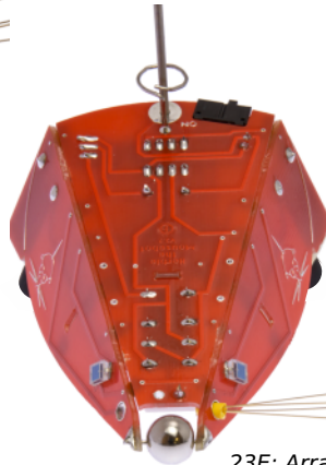
23E: Arrange the sensors so they stick straight out the side of Herbie
