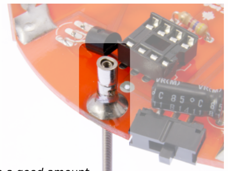
13C: Use a good amount of solder to mount the tail
