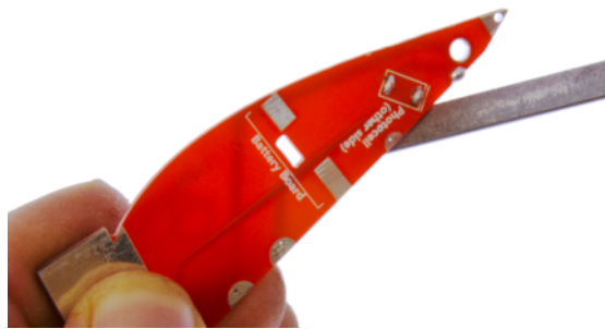
1B. Filing down the tab grooves
