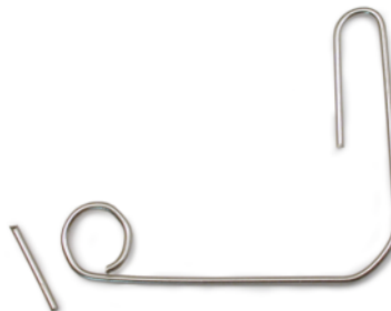
14C: Turn one end into a loop and snip the extra wire off
