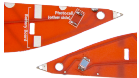
2B. Photocells soldered in flat against PCB
