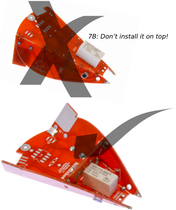
7C: Installed, nice and flat
