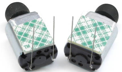
16C: Solder on wire clippings
