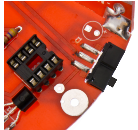
11B: Switch soldered in place
