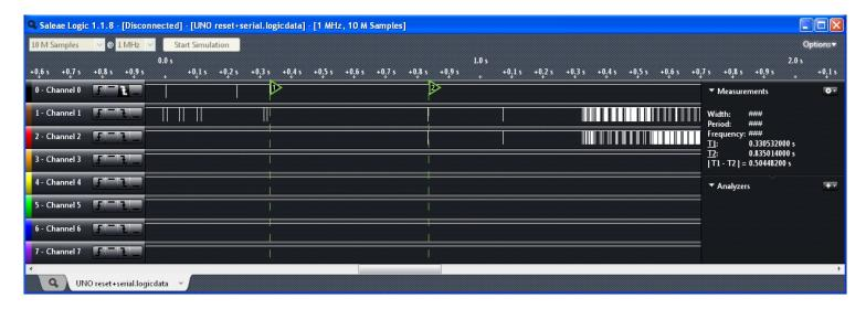
The measurement of 1S represents the 1S reset delay that we programmed into the Synapse node.
