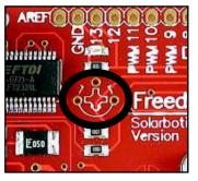
We suggest installing a 10k or 100k trimpot (our part RT10k or RT100k) to set your new desired ARef (between 0 and 5 volts). Set the new voltage by measuring the AREF pin (up top, next to the GND pin).
