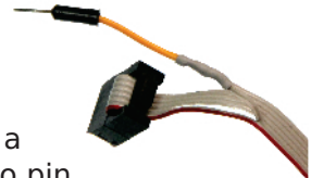
Arduino-as-ISP trick needs a hacked cable
