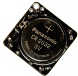
Battery installed. Make sure it snaps in!
