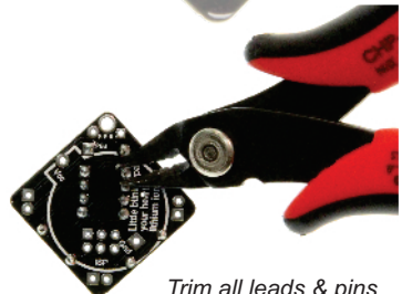
Trim all leads & pins on the PCB underside
