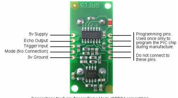
Connections for 2-pin Trigger/Echo Mode (SRF04 compatible)
