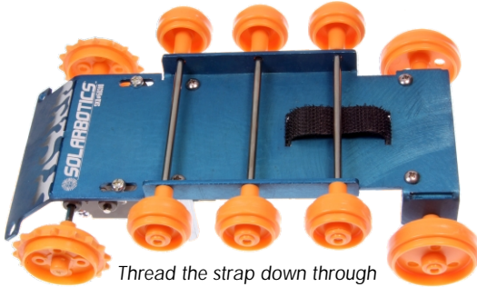
Thread the strap down through the slot, and back up through the other
