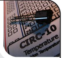
degree centigrade on the signal pin (to allow measuring temperatures below freezing there is a 500 mV offset eg.  $25^{\circ}$  C = 750 mV,  $0^{\circ}$  C = 500mV). To convert this from the digital value to degrees, we will use some of the Arduino's maths abilities. Then to display it we'll use one of the IDE's rather powerful features, the debug window. We'll output the value over a serial connection to display on the screen. Let's get to it.
