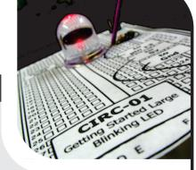
everything in. Once the circuit is assembled you'll need to upload the program. To do this plug the Arduino board into your USB port. Then select the proper port in **Tools > Serial Port > (the** comm port of your Arduino). Next upload the program by going to File > Upload (ctrl+U). Finally, bask in the glory and possibility that controlling lights offers.
