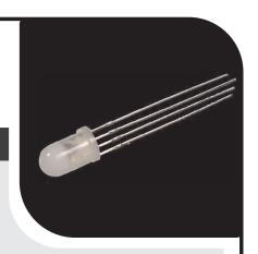
The RGB LED actually has 3 LED elements inside it - Red, Green & Blue. Let's turn these on in combinations to get some brilliant colours out of a single LED!
