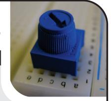
it to a digital number between 0 (0 volts) and 1023 (5 volts) (10 bits of resolution). A very useful device that exploits these inputs is a potentiometer (also called a variable resistor). When it is connected with 5 volts across its outer pins the middle pin will read some value between 0 and 5 volts dependent on the angle to which it is turned (ie. 2.5 volts in the middle). We can then use the returned values as a variable in our program.
