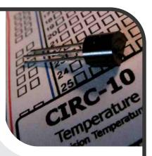
degree centigrade on the signal pin (to allow measuring temperatures below freezing there is a 500 mV offset eg. 25° C = 750 mV, 0° C = 500mV). To convert this from the digital value to degrees, we will use some of the Arduino's maths abilities. Then to display it we'll use one of the IDE's rather powerful features, the debug window. We'll output the value over a serial connection to display on the screen. Let's get to it.
