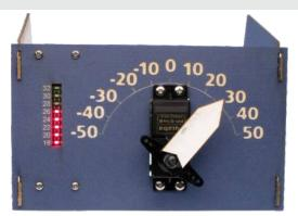
Dual-Temperature display using Ardweeny Backpack's Servo-output, LED bargraph, and TMP36 temperature sensor. Get source-code from our website!
