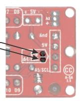
The SMD LEDs on the bottom of the SMD-versions of the BackPack can be each (or globally) disabled by cutting the trace connected to the LED just above each of the "Dx" lables.
