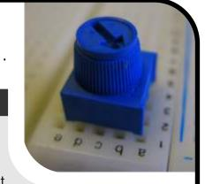
it to a digital number between 0 (0 volts) and 1024 (5 volts) (10 bits of resolution). A very useful device that exploits these inputs is a potentiometer (also called a variable resistor). When it is connected with 5 volts across its outer pins the middle pin will read some value between 0 and 5 volts dependent on the angle to which it is turned (ie. 2.5 volts in the middle). We can then use the returned values as a variable in our program.
