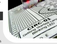
everything in. Once the circuit is assembled you'll need to upload the program. To do this plug the Arduino board into your USB port. Then select the proper port in Tools > Serial Port > (the comm port of your Arduino). Next upload the program by going to File > Upload to I/O Board (ctrl+U). Finally, bask in the glory and possibility that controlling lights offers.
