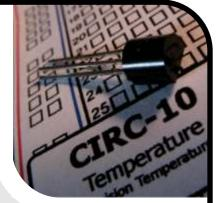
degree centigrade on the signal pin (to allow measuring temperatures below freezing there is a 500 mV offset eg.  $25^{\circ}$  C = 750 mV,  $0^{\circ}$  C = 500mV). To convert this from the digital value to degrees, we will use some of the Arduino's maths abilities. Then to display it we'll use one of the IDE's rather powerful features, the debug window. We'll output the value over a serial connection to display on the screen. Let's get to it.
