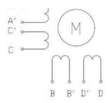
Two-phase unipolar stepper motor with eight leads.
