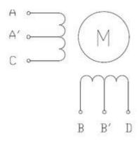
Two-phase unipolar stepper motor with six leads.
